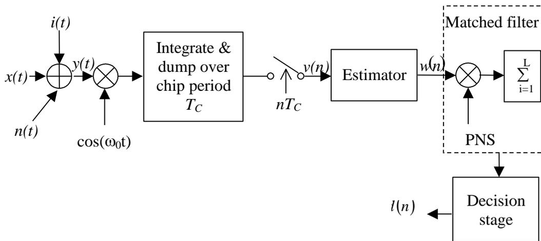
Fig.2 The DS-SS receiver structure based on estimator application
