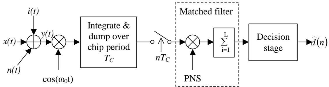
Fig.1 The DS-SS receiver structure based on simple MF
