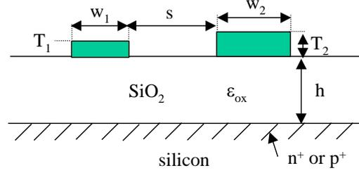
**Fig. 2** The interconnect lines in a VLSI chip
