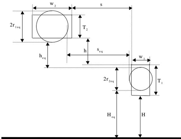
**Fig. 1** Two rectangular conductors over a single ground plane and capacitance definitions (cross-section)
