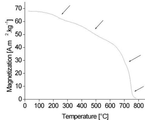
**Fig. 3** Thermomagnetic curve of the sample after 550 hours of milling.
