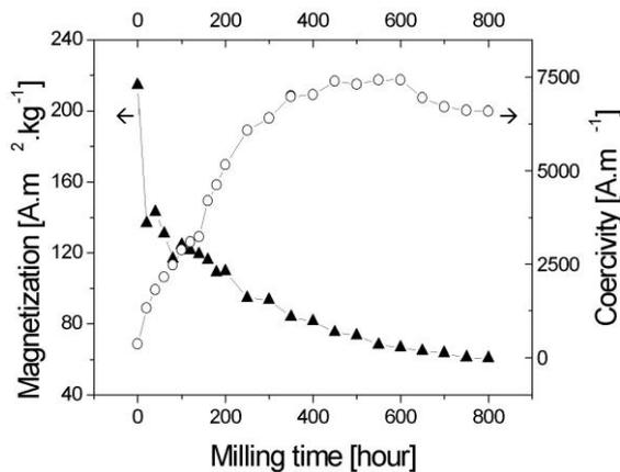
**Fig. 1** Magnetization and coercivity of the Fe-Si alloy vs. milling time.
