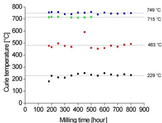
**Fig. 4** Curie temperatures of the Fe-Si phases for the samples after different stages of milling.
