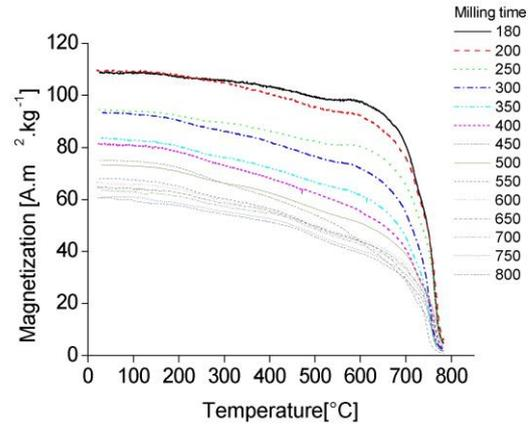
**Fig. 2** Thermomagnetic curves for different stages of milling.
