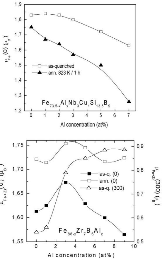
**Fig. 3** Concentration dependence of the magnetic moment per magnetic atom in the investigated alloys in as-quenched state and after annealing.
