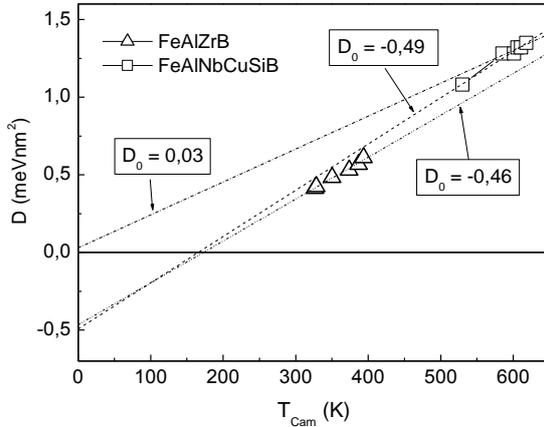
**Fig. 2** Relationship between the spin-wave stiffness constant and the Curie temperature in the investigated as-quenched samples.
