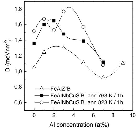
**Fig. 4** Concentration dependence of the spin-wave stiffness constant for the annealed samples.
