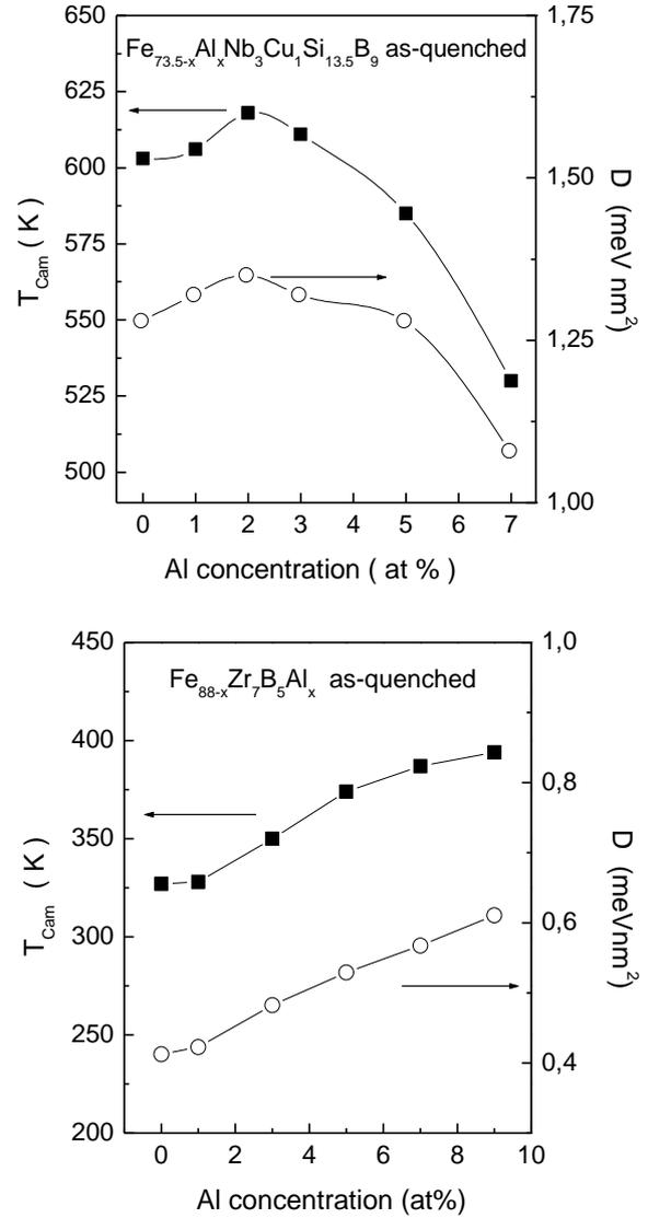
**Fig. 1** Concentration dependence of the spin-wave stiffness constant and the Curie temperature of the investigated as-quenched alloys.
