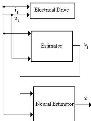
Fig. 4 Neural networks structure estimation of angular speed
