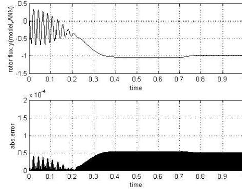
Fig. 2 Course of the flux component  $\psi_{2y}$  and the absolute error
