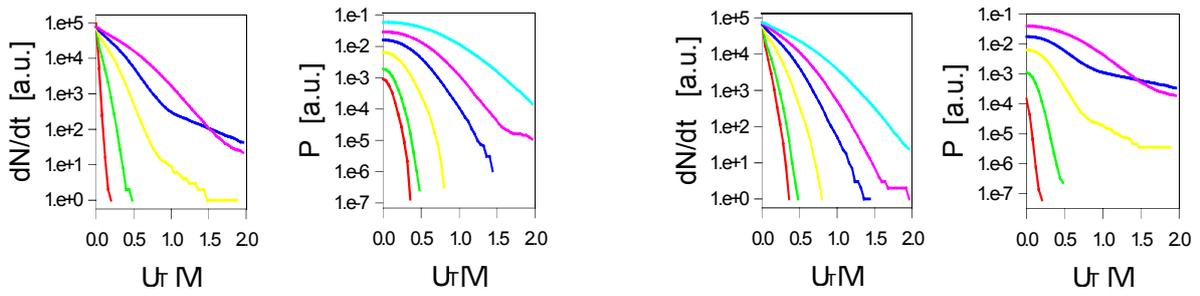
**Fig. 4** Calculated amplitude distribution families of AE impulses registered at measuring points P3 (a, b) and P5 (c, d)
