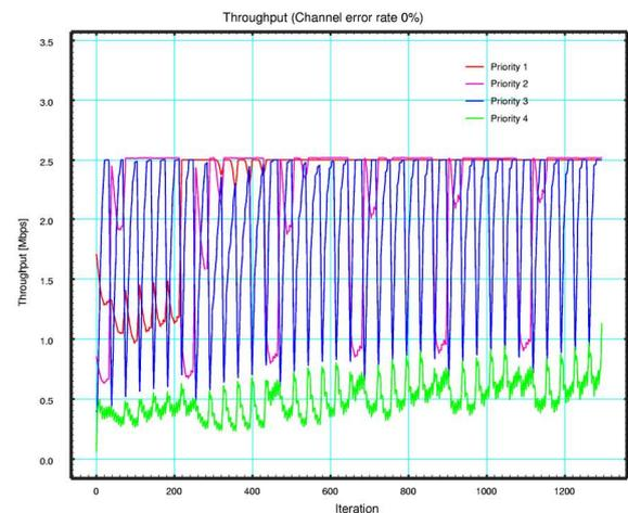
Fig. 3 Throughput of the 4 traffic classes in relation to the packet size combination iteration, when the channel error rate is 0%
