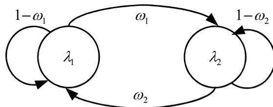
Fig. 1 State machine for a 2-state MMPP
