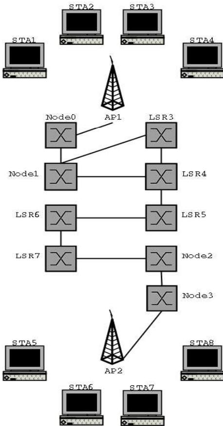
**Fig. 8** End-to-end network simulation configuration
