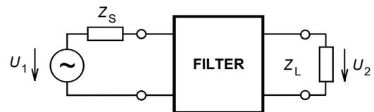
**Fig. 1** Basic EMI filter setup
