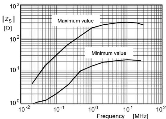
**Fig. 3** Powerline HF impedance of commercial European power lines [3]
