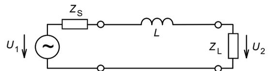
Fig. 5 Basic form of an L-filter.
