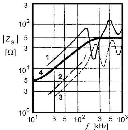
**Fig. 2** HF impedance of various types of power line networks (1 – outdoor distribution network; 2 – industrial distribution network; 3 – cable earth distribution network; 4 – CISPR specification [2])
