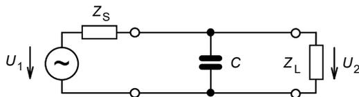
Fig. 4 Basic form of a C-filter
