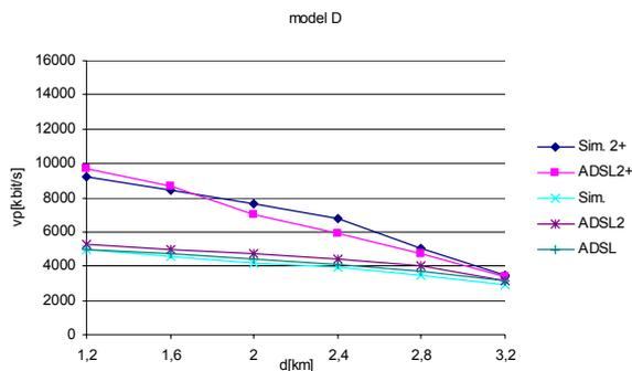
**Fig. 3** Comparison of simulation results with measured speeds
