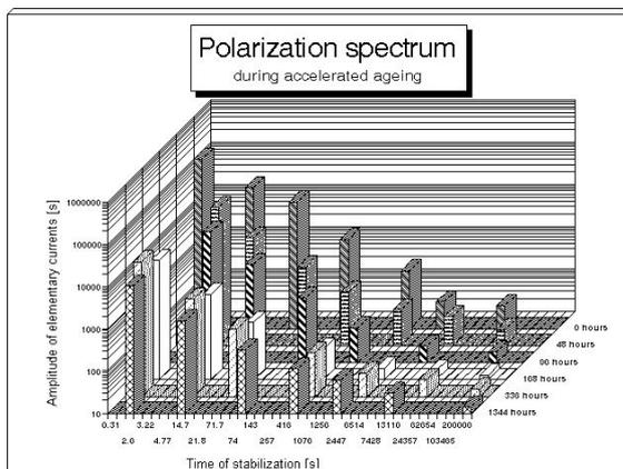
Fig. 4 Polarization spectrum during accelerated thermal stress
