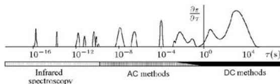
**Fig. 1** Common polarization spectrum of insulation material
