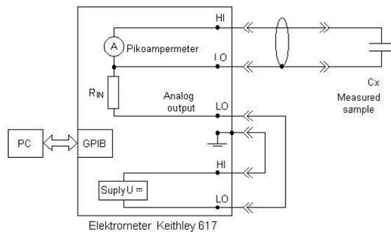
Fig. 3 Scheme for measuring of absorptive current of sample
