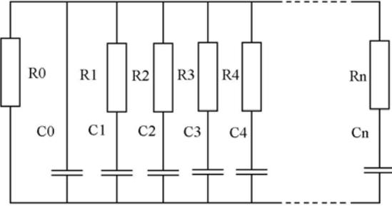
Fig. 2 Maxwell - Wagner equivalent model
