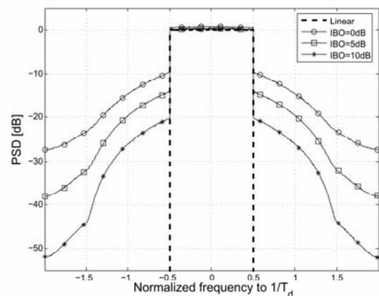
Fig. 6 PSD of the signal at the input and the output of the nonlinearity.
