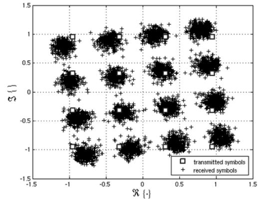
Fig. 5 Original and received signal constellation.
