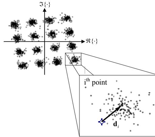
Fig. 7 Definition of Target Error Vector (TEV).
