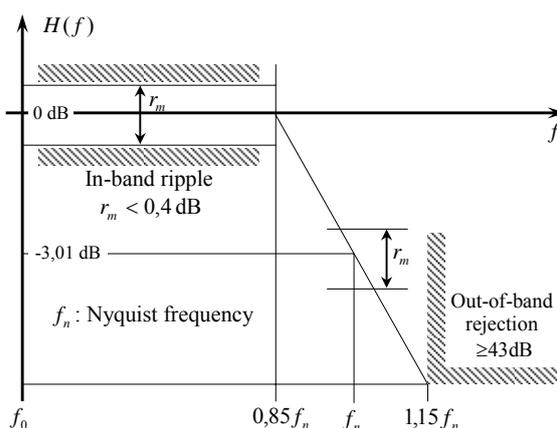
Fig. 8 Spectrum mask for out-of-band emission measurement.
