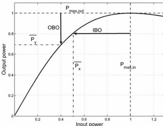
**Fig. 4** Graphical representation of IBO and OBO.
