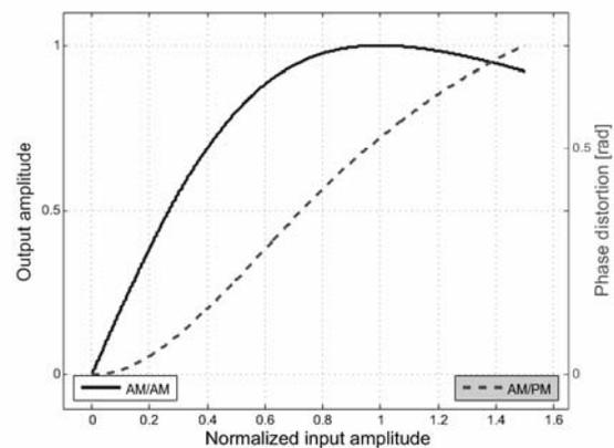
**Fig. 2** AM/AM and AM/PM characteristics of the normalized Saleh model.
