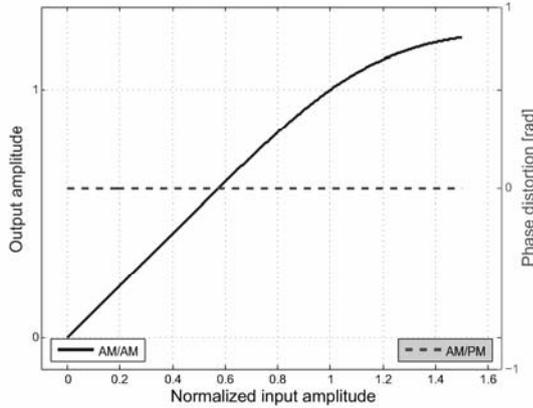
**Fig. 3** AM/AM and AM/PM characteristics of the normalized Rapp model
