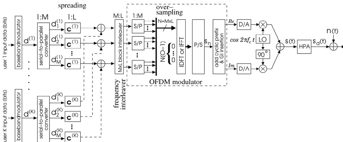
Fig. 1 The block diagram of an MC-CDMA synchronous downlink transmitter.
