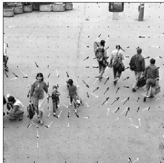
Fig. 1 The frame from the image sequence "Railway station" with motion vectors founded by FS method (white) and 2Dlog method (black)
