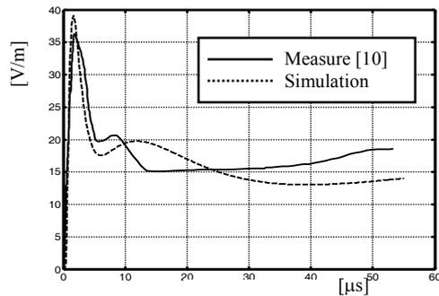
Fig. 4 Calculated and measured vertical electric field
