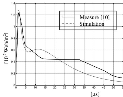
**Fig. 3** Calculated and measured magnetic flux densities
