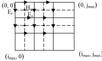
Fig. 7 2D-FDTD Meshes of cylindrical coordinates
