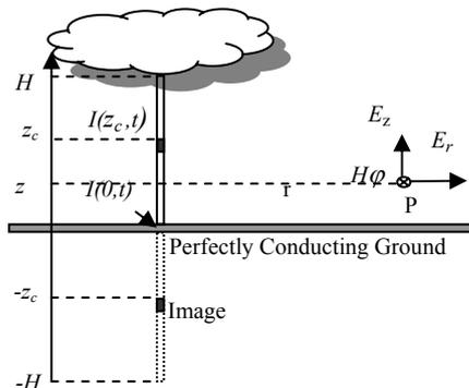
Fig. 1 Lightning channel geometry
