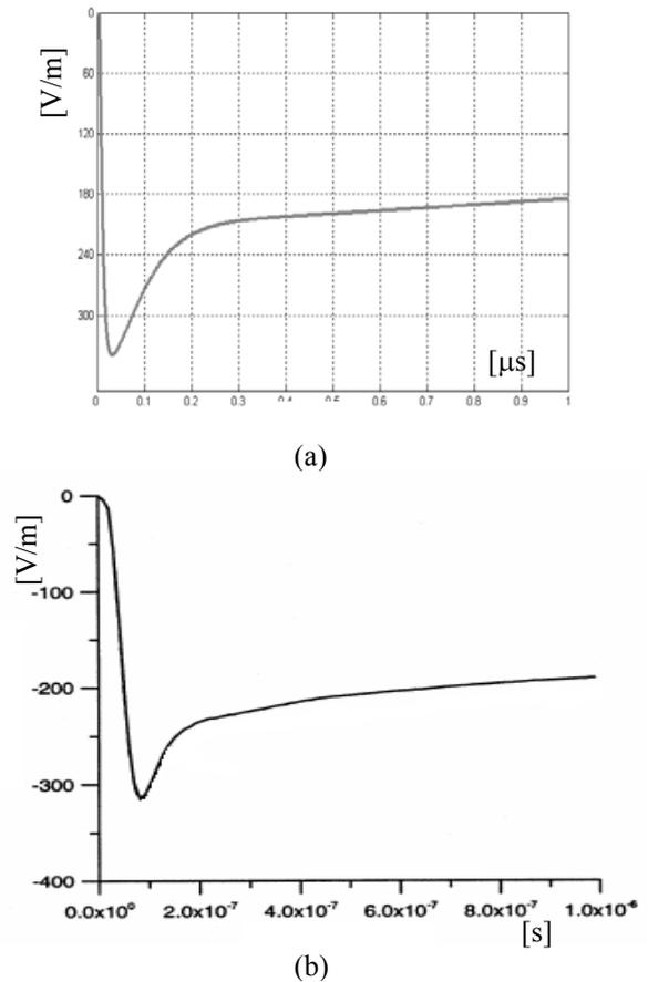
**Fig. 10** Computed horizontal electric field at ground level and distance of 100 m. ( $\sigma=0.01$  S/m)
