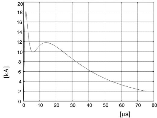
**Fig. 2** Lightning channel base current waveshape
