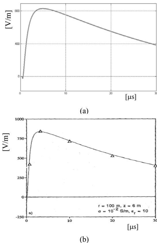
**Fig. 9** Horizontal electric field (a) Using the quasi-FDTD method, (b) Adopted from [12]
