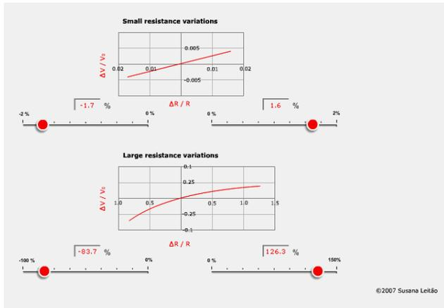
Fig. 8 The transfer function of a Wheatstone bridge
