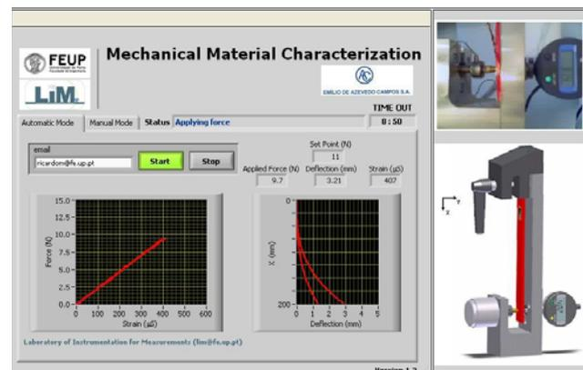
**Fig. 3** User interface in automatic operation mode
