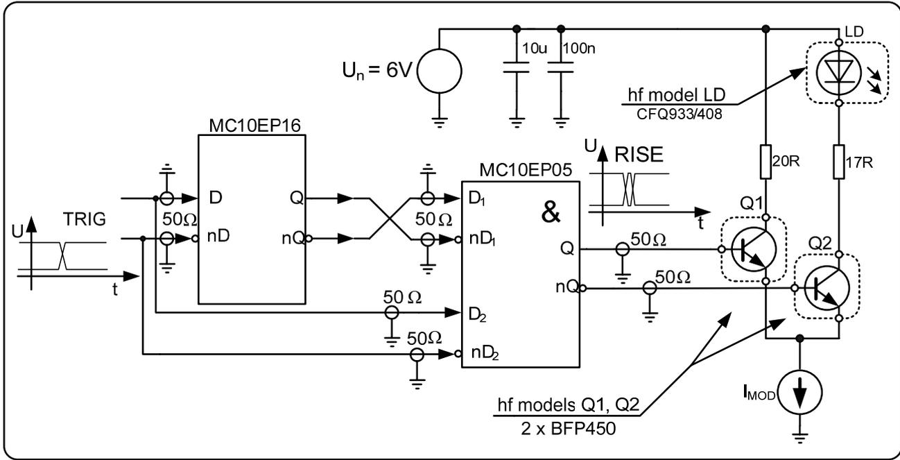
Fig. 6 Simulation model
