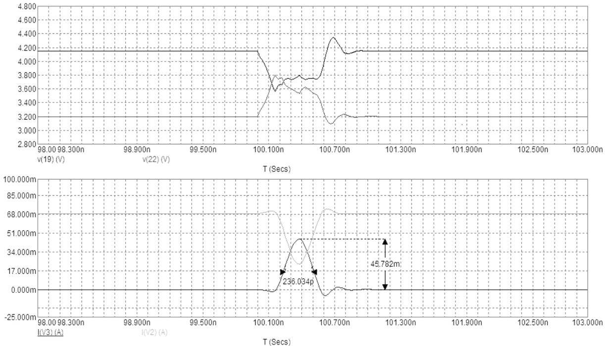
Fig. 7 Time analyze simulation of final stage
