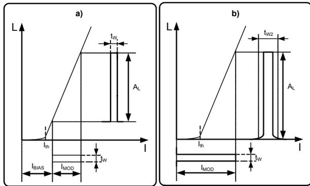
Fig. 3 a/b Types of modulation in PC-OTDR
