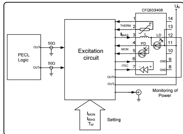
Fig. 2 The excitation circuit scheme
