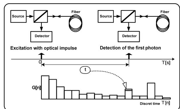
Fig. 1 The principle of PC-OTDR histogram forming [1]
