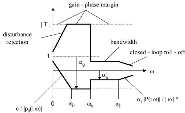
**Fig. 1** Requirement envelope for robust control design in frequency domain
