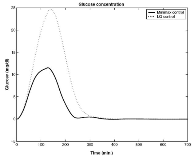
**Fig. 3** Blood glucose concentration,  $G(t)$  for LQ and “modified” minimax control
