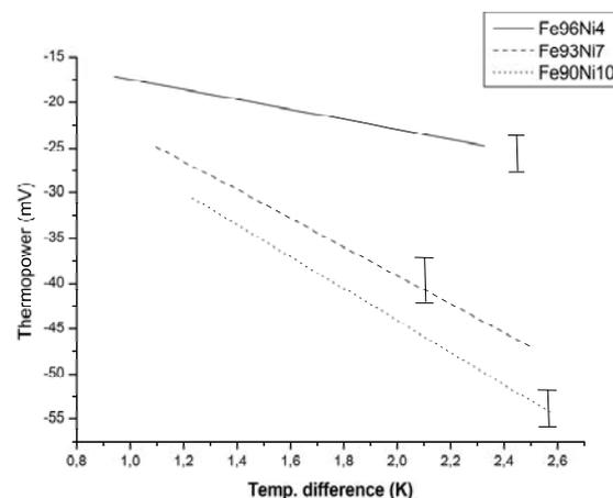
**Fig. 4** Thermoelectric power of  $\text{Fe}_x\text{Ni}_{1-x}$  alloys after slow cooling
