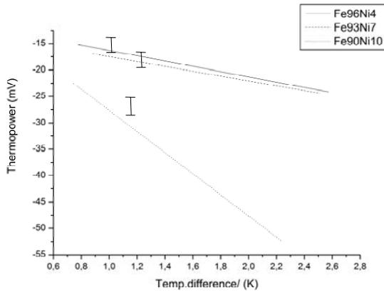
Fig. 5 Thermoelectric power of  $\text{Fe}_x\text{Ni}_{1-x}$  alloys after quenching (water quenching)
