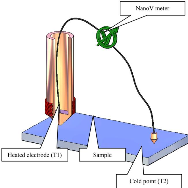
**Fig. 1** The principle of the TEP measurement and the scheme of the experimental setup
