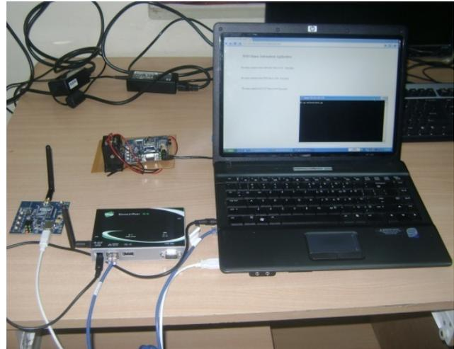
Fig. 1 DIGI ZigBee mesh network kit
