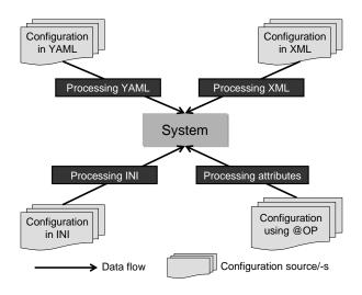
Fig. 1 Example of Ad-hoc solution with four configuration languages
