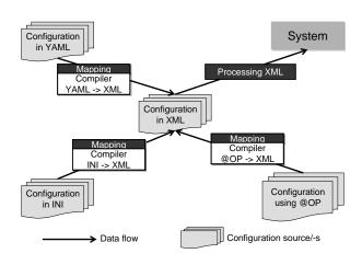
Fig. 2 Example of source transformations with four configuration languages
