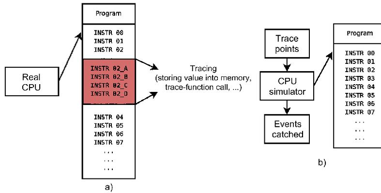
Fig. 2 Typical approaches to dynamic timing analysis: a) code tracing, b) code simulation
