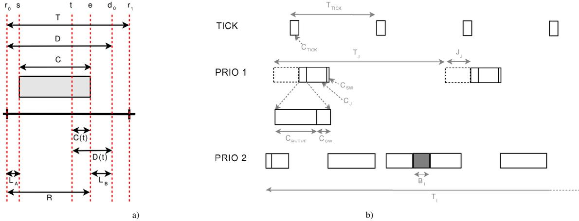
**Fig. 1** Illustration to a) RT task parameters and b) extended version of a formula for  $R_i$  enumeration
