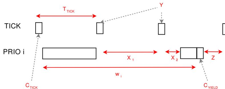
Fig. 5 Illustration to parameters for  $R_i$  enumeration of FreeRTOS tasks
