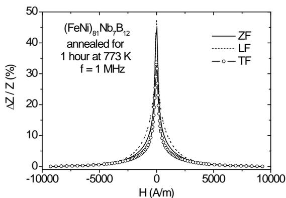
**Fig. 4** Magnetic field dependence of GMI ratio  $\Delta Z/Z$  after different field annealing for nanocrystalline  $(\text{Fe}_{0.5}\text{Ni}_{0.5})_{81}\text{Nb}_7\text{B}_{12}$
