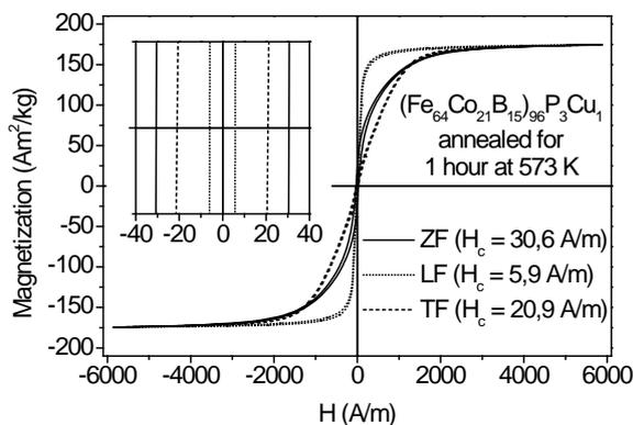
**Fig. 2** Hysteresis loops for  $(\text{Fe}_{63}\text{Co}_{21}\text{B}_{15})_{96}\text{P}_3\text{Cu}_1$  after different field annealing for 1 hour at 573 K, zero field annealing (ZF), longitudinal field annealing (LF) and transverse field annealing (TF)
