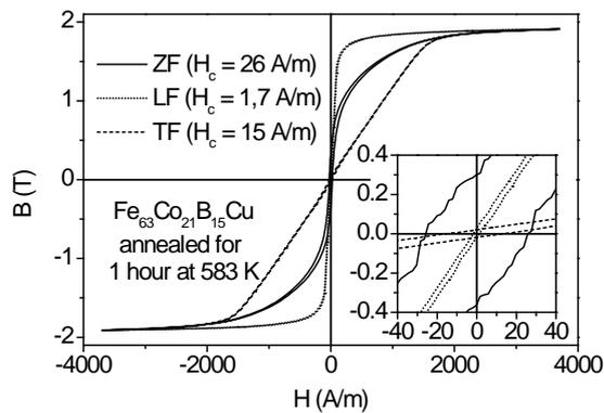
**Fig. 1** Hysteresis loops for  $\text{Fe}_{63}\text{Co}_{21}\text{B}_{15}\text{Cu}$  after different field annealing for 1 hour at 583 K, zero field annealing (ZF), longitudinal field annealing (LF) and transverse field annealing (TF)
