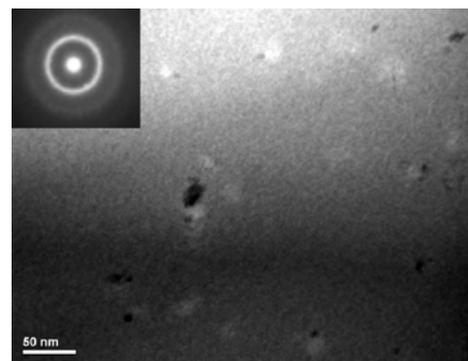
**Fig. 6** TEM micrograph of  $\text{Gd}_{65}\text{Fe}_{20}\text{Al}_{10}\text{B}_5$  melt-spun ribbon in the as-quenched state
