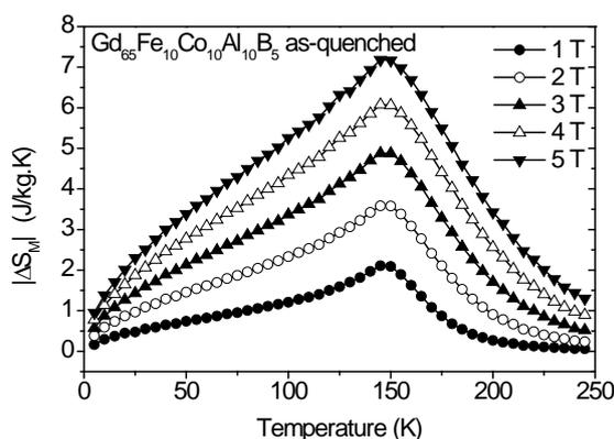
**Fig. 8** The magnetic entropy changes  $|\Delta S_M|$  vs. temperature T calculated for different changes of external magnetic field  $\Delta H$  up to 5T
