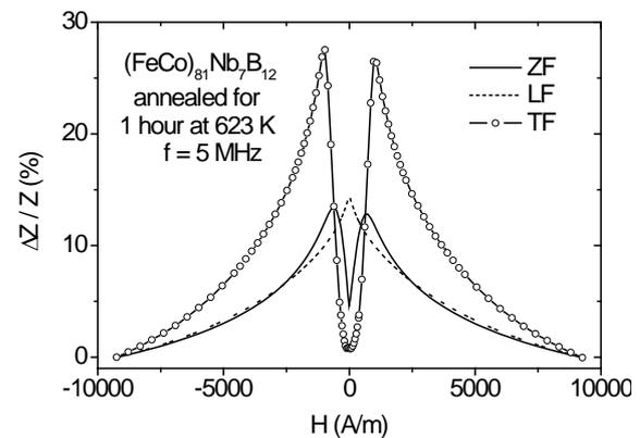
**Fig. 5** Magnetic field dependence of GMI ratio  $\Delta Z/Z$  after different field annealing for amorphous  $(\text{Fe}_{0.5}\text{Co}_{0.5})_{81}\text{Nb}_7\text{B}_{12}$
