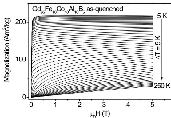
**Fig. 7** Field dependences of the magnetization measured at 5K steps
