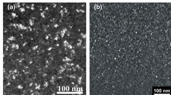
**Fig. 3** TEM micrographs of nanocrystalline samples annealed at 773 K.  $(\text{Fe}_{0.5}\text{Co}_{0.5})_{81}\text{Nb}_7\text{B}_{12}$  (a) and  $(\text{Fe}_{0.5}\text{Ni}_{0.5})_{81}\text{Nb}_7\text{B}_{12}$  (b)
