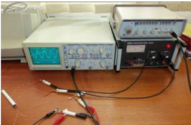
Fig. 4 Experimental workplace for GMI measurement
