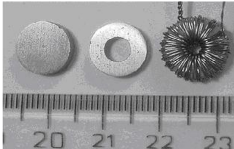
Fig. 2 Bulk samples \text{Ni}_{81}\text{Fe}_{19} (wt.%) prepared for ac and dc measurements
