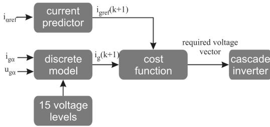
Fig. 2 Predictive current controller of cascade inverter
