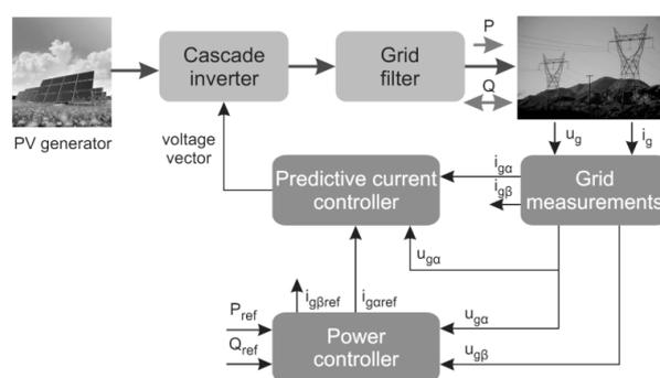
Fig. 1 Proposed control scheme for power control flow of grid connected cascade inverter
