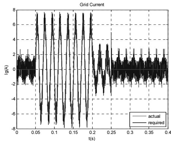
**Fig. 10** Comparison of required and actual grid current for  $L = 2$  mH
