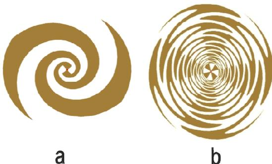
**Fig. 2** Two arms spiral antenna (a), sinuous antenna (b)
