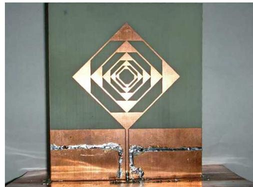
Fig. 8 UWB fractal antenna with five iterations [15]
