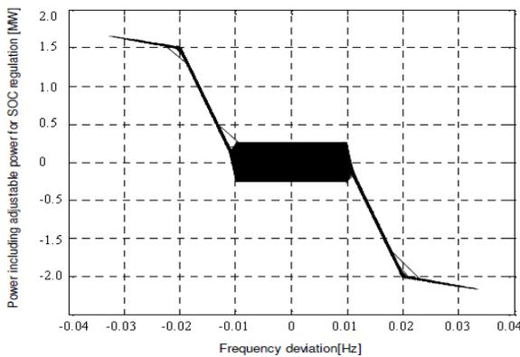
Fig. 3 Power-frequency characteristic having
