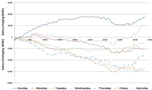
Fig. 4 SOC level as a function of time for week
