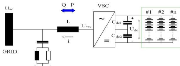
Fig. 1 Schematic layout of STATCOM with Energy Storage
