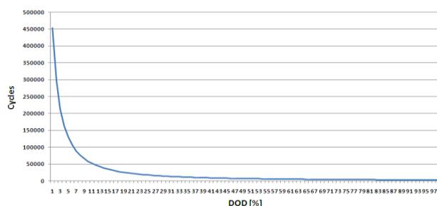
Fig. 6 Cycle-life curve for the lithium-ion battery system
