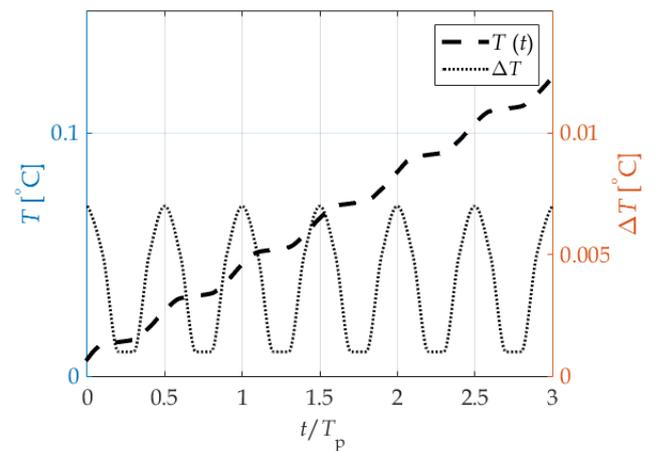
Fig. 5 Time evolution of increments of temperature  $\Delta T(t)$  and average temperature  $T(t)$  of conductor X
