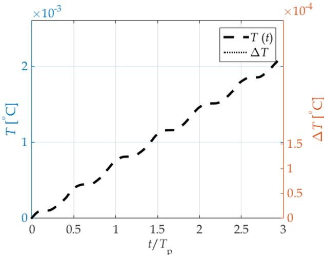
**Fig. 7** Time evolution of increments  $\Delta T(t)$  and average temperature  $T(t)$  of shielding shell of conductor X
