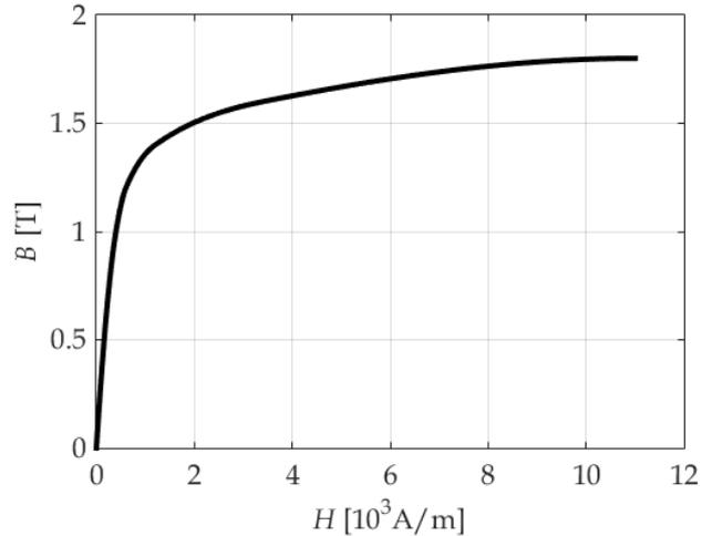
**Fig. 3** Magnetization curve of the steel used for shielding
