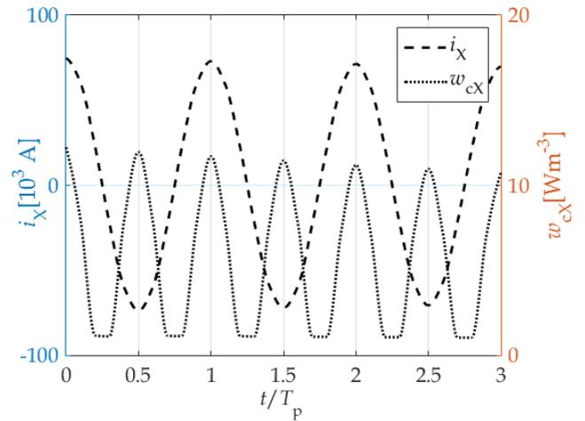
Fig. 4 Average value of the volumetric Joule losses  $w_{cX}(t)$  caused by the short-circuit current  $i_X(t)$
