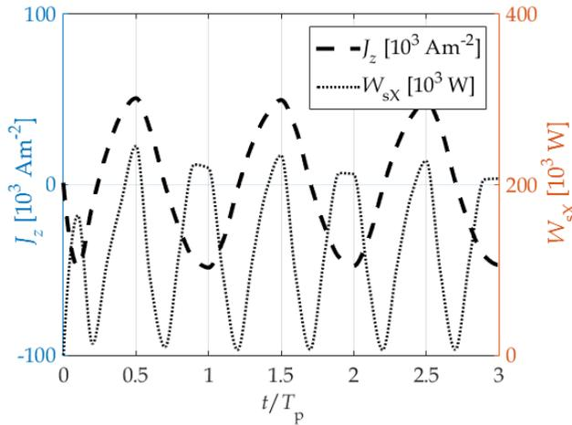
**Fig. 6** Average values of eddy current densities  $J_z$  and corresponding average value of Joule losses  $W_{sX}(t)$  in shielding of conductor X
