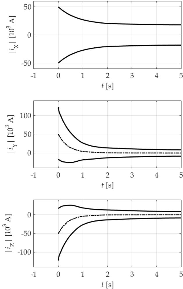
**Fig. 2** Time evolution of amplitudes of short-circuit currents  $i_X$ ,  $i_Y$ ,  $i_Z$
