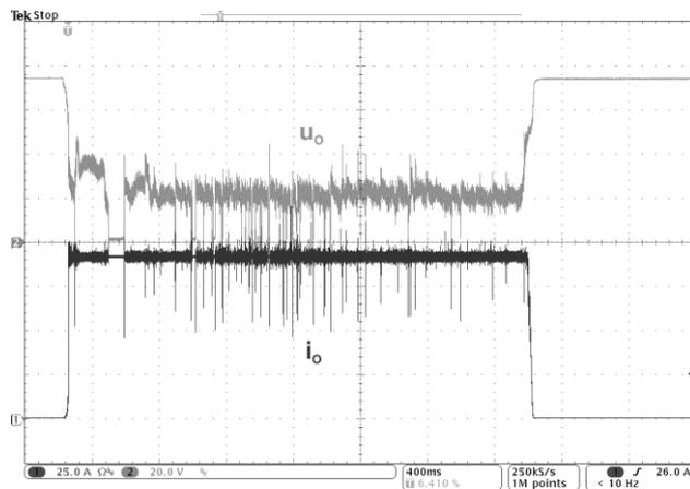
Fig. 13 Output voltage  $u_o$  and output current  $i_o$  during welding at output current of 90 A
