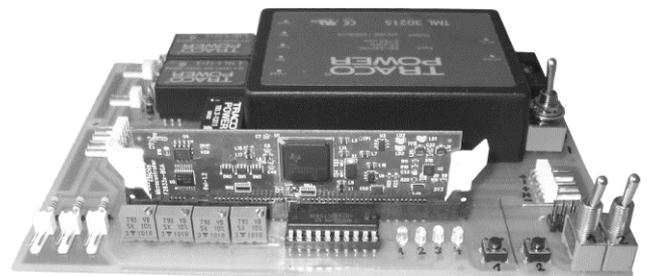
Fig. 7 Basic control board with TMDSCNCD28335 card
