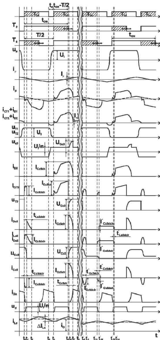
Fig. 2 Converter waveforms for rated load (left side) and light load (right side)
