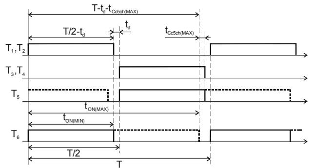
Fig. 4 Control pulses for the converter
