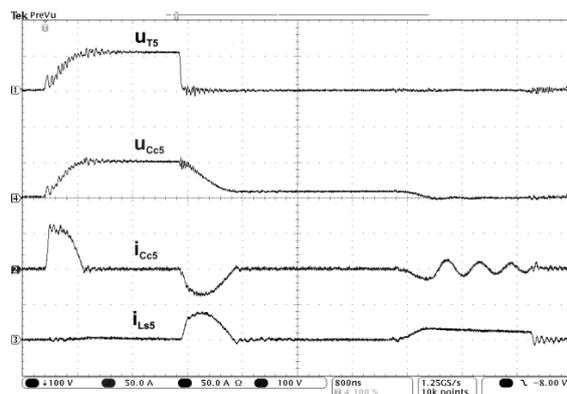
**Fig. 12** Drain-source voltage  $u_{T5}$ , snubber capacitor voltage  $u_{Cc5}$  and current  $i_{Cc5}$  and snubber inductor current  $i_{Ls5}$  at light load
