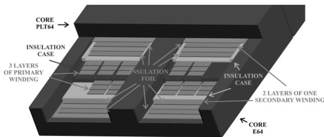
**Fig. 9** Power planar transformer arrangement
