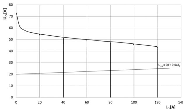
Fig. 14 Measured output characteristics of the welder
