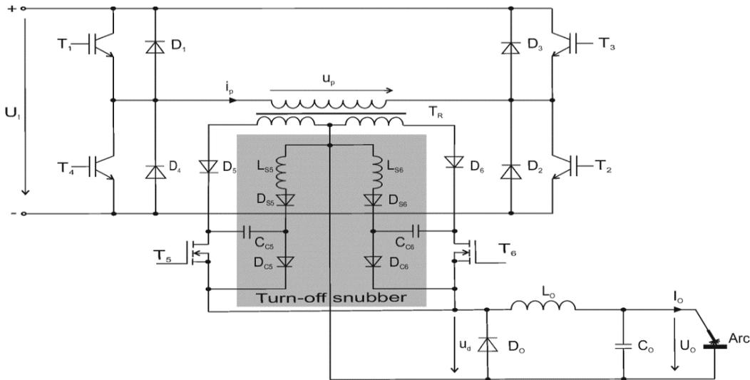
Fig. 1 ZVZCS PWM DC-DC power converter
