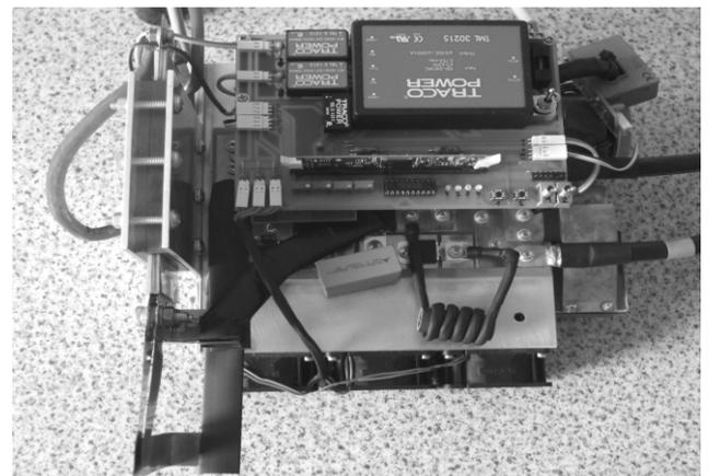
Fig. 8 Laboratory model of the converter
