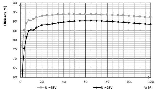
Fig. 15 Measured efficiency of the converter
