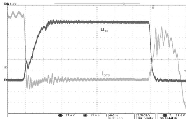
**Fig. 11** Drain-source voltage  $u_{T5}$  and drain current  $i_{DT5}$  of secondary transistor  $T_5$
