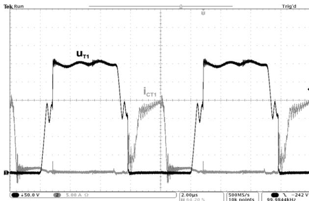
**Fig. 10** Collector-emitter voltage  $u_{T1}$  and collector current  $i_{CT1}$  of primary transistor  $T_1$
