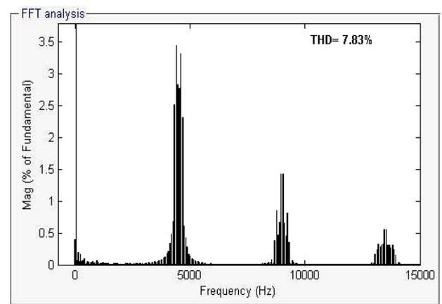
**Fig. 13** THD analysis of stator current
