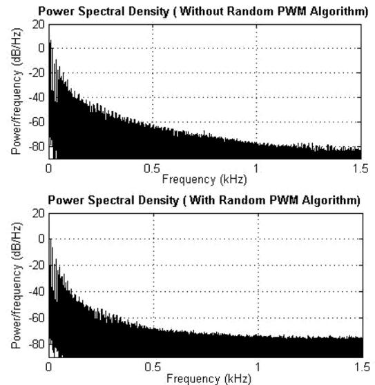
Fig. 24 Acoustic noise Comparison without and with random PWM Algorithm
