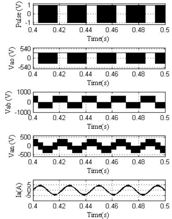
**Fig. 12** Pulses, Pole voltage, Line voltage, Phase voltage and stator current
