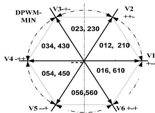
Fig. 5 Voltage space vectors for DPWMMIN
