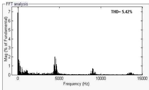
Fig. 22 THD analysis of stator current
