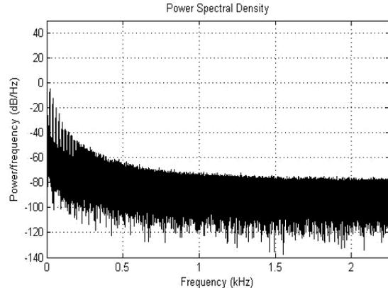
**Fig. 20** Acoustic noise for VDR DPWMIN
