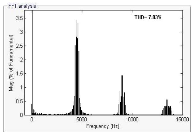
**Fig. 13** THD analysis of stator current
