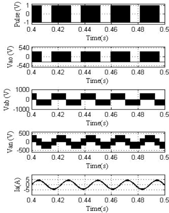
**Fig. 9** Pulses, Pole voltage, Line voltage, Phase voltage and stator current
