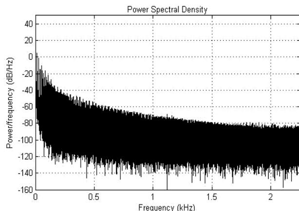
**Fig. 8** Acoustic noise for SVPWM
