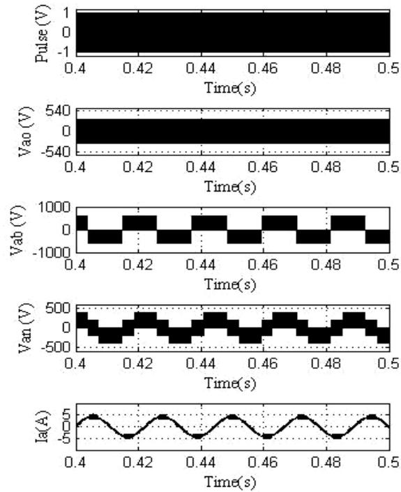
**Fig. 6** Pulses, Pole voltage, Line voltage, Phase voltage and stator current
