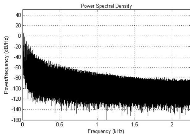
**Fig. 8** Acoustic noise for SVPWM
