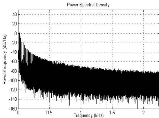
**Fig. 11** Acoustic noise for DPWMMIN
