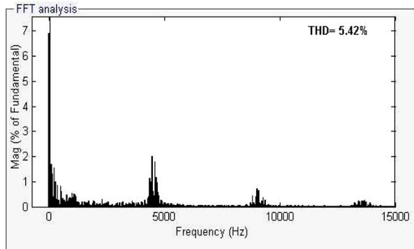
Fig. 22 THD analysis of stator current
