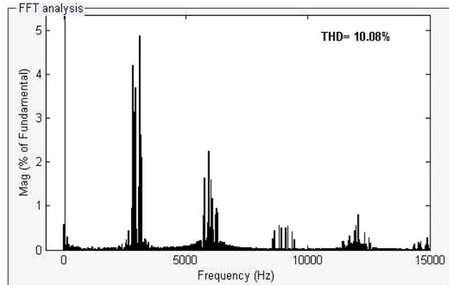
**Fig. 7** THD analysis of stator current
