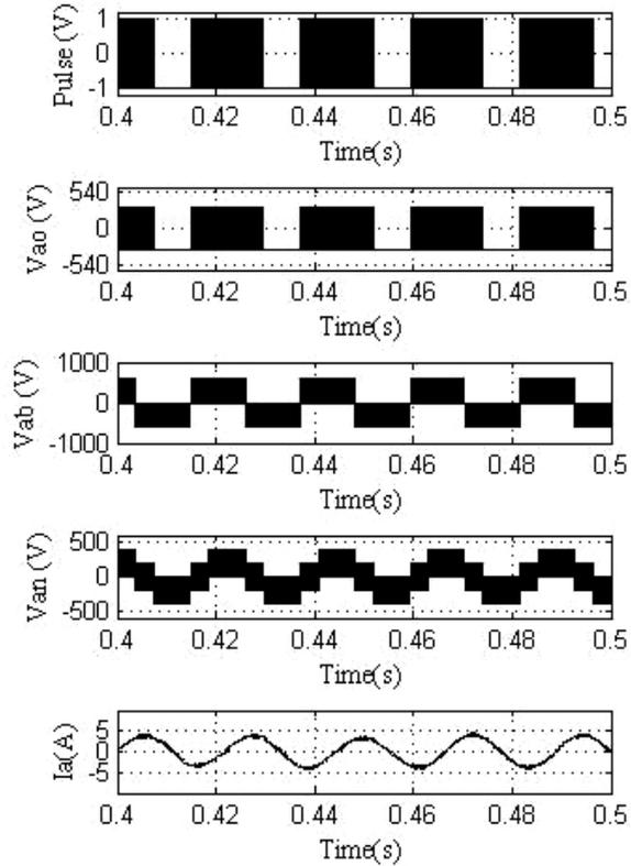
**Fig. 15** Pulses, Pole voltage, Line voltage, Phase voltage and stator current
