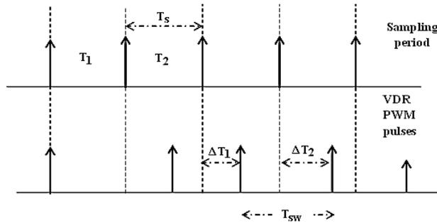
Fig. 2 Timing diagram for VD-RPWM implementation
