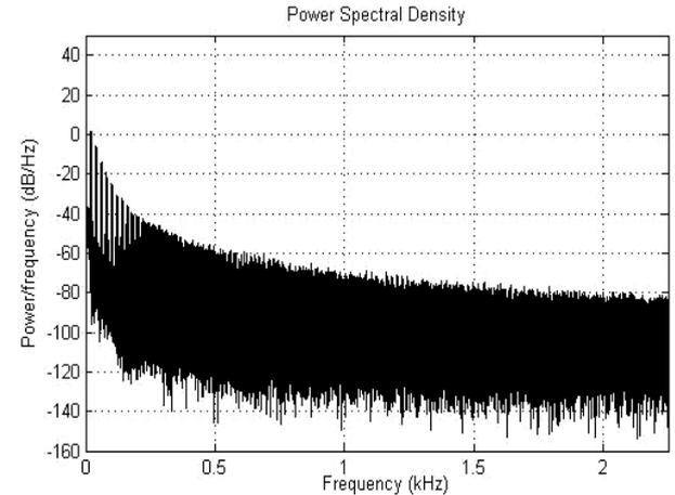
**Fig. 14** Acoustic noise for DPWMMAX
