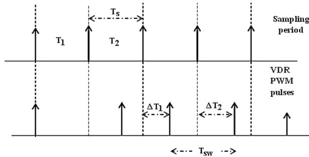
Fig. 2 Timing diagram for VD-RPWM implementation
