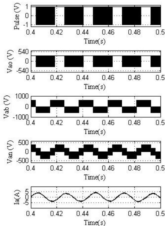
Fig. 21 Pulses, Pole voltage, Line voltage, Phase voltage and stator current
