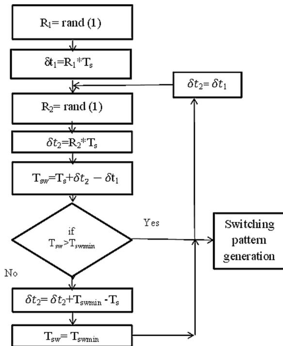
Fig. 3 Flow chart of a VDPWM algorithm
