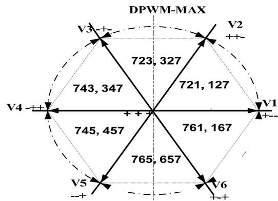
Fig. 4 Voltage space vectors for DPWMMAX
