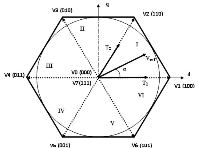
Fig. 1 Voltage space vectors for SVPWM
