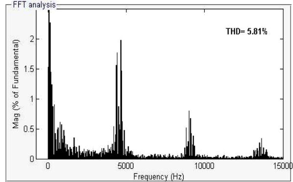
**Fig. 16** THD analysis of stator current
