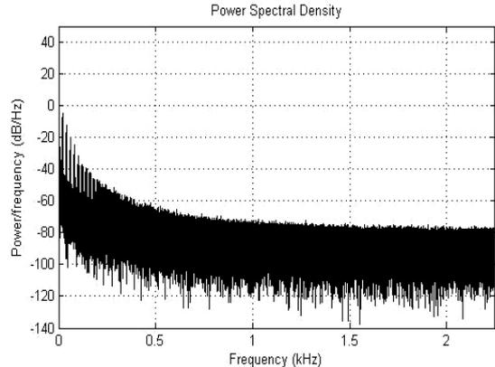
**Fig. 20** Acoustic noise for VDR DPWMIN
