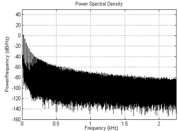
**Fig. 14** Acoustic noise for DPWMMAX
