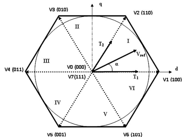
Fig. 1 Voltage space vectors for SVPWM
