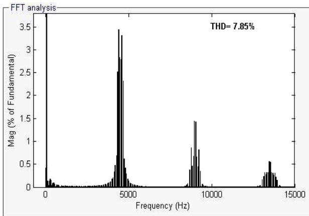
**Fig. 10** THD analysis of stator current
