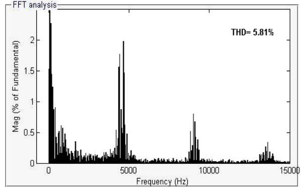
**Fig. 16** THD analysis of stator current
