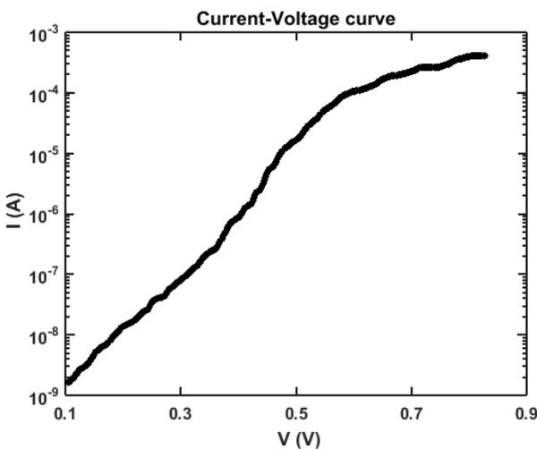
**Fig. 3** Plot of  $I$ - $V$  curve of experimental data of Au/ $n$ GaAs Schottky diode taken from [17]. The original curve of [17] was redrawn and digitized with an interval of 2 mV.
