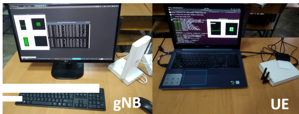
Fig. 2 Experimental testbed of the virtualized 5G network based on software defined radio
