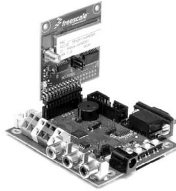
Fig. 7 The DEMC ADuC BOARD with x51 core micro-converter with inserted Freescale RF board
