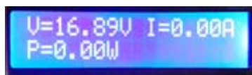
Fig. 9 A capture of the readings on LCD screen when no load was connected
